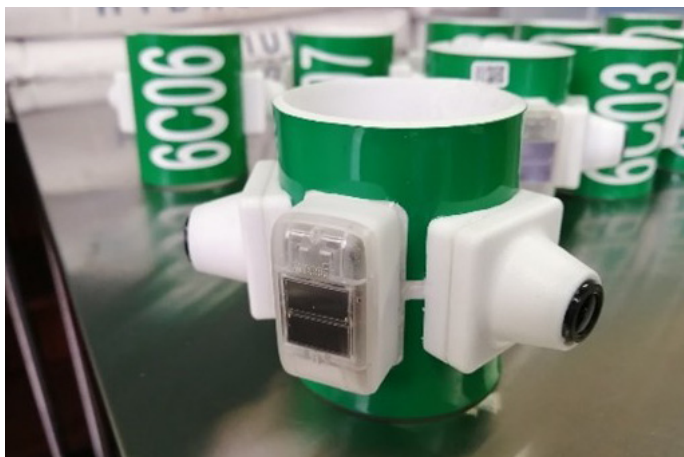
Figure 1: GPS logger with camera (SwanEyes). The square in the center is the GPS unit, flanked by two cameras positioned at a 60-degree angle, providing a 240-degree field of view. The total weight is 130g.
